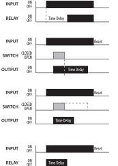
see TGL, pg 138 with wired connection between T1 and T2, delay starts with Power On and de-energizes at end of time delay. Resets with Power Off.
